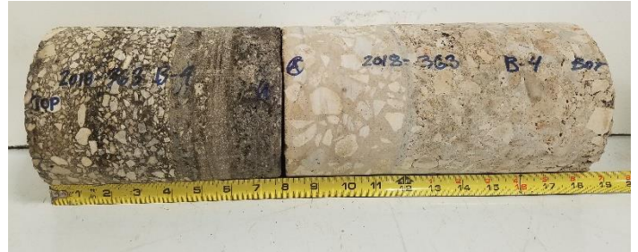
Asphalt and Concrete Core from Boring B-4 North of Broadway St and E. Mulberry Ave. Intersection At Southbound Left Turn Lane to E. Mulberry Ave.
