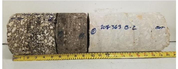
Asphalt and Concrete Core from Boring B-2 North of Broadway St and Pershing Ave. Intersection At Southbound Left Turn Lane to Pershing Lane
