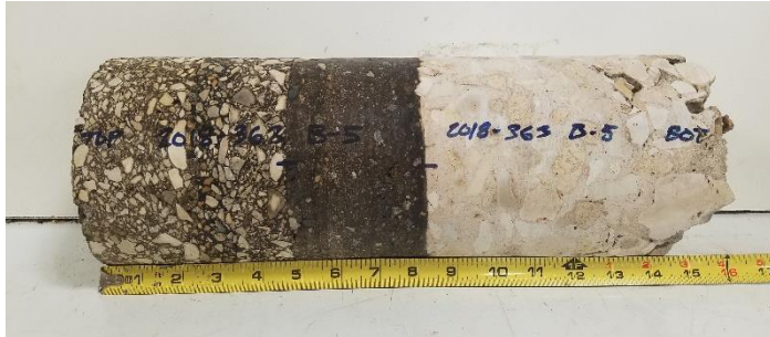
Asphalt and Concrete Core from Boring B-5 North of Broadway St and Post Ave. Intersection At Southbound Left Lane
