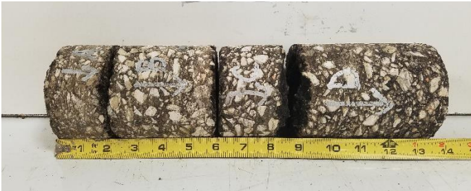
Asphalt Core from Boring B-1 North of Broadway St and Groveland Pl Intersection At Median between Northbound and Southbound Broadway St
